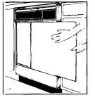
Special 1/4" thick wood inserts can replace the two metal panels. Dimensions for ¼" wood inserts: Door Panel: 23 ¼"W x 16¹¼6"H. Access Panel: 23 ¼"W x 6½"H.
